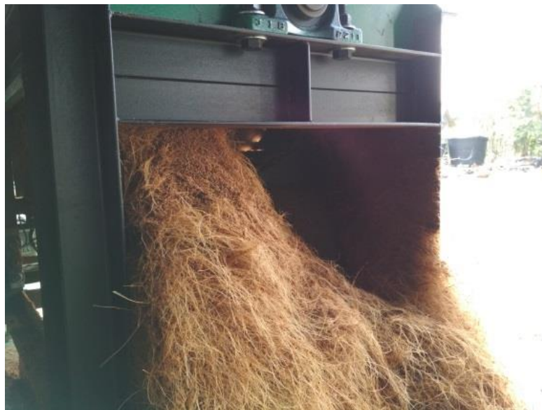
Figure 10. Extracted fiber before screening process.
