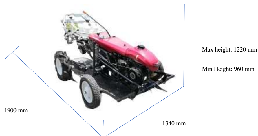
Figure 1. Overall view of the PHI-A pedestrian-type vegetables transplanter.
