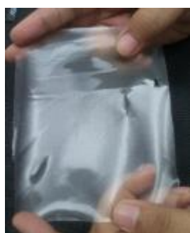
Figure 3. Plasticized starch-based film without lemongrass oil.
