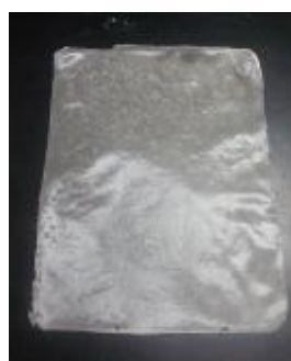
Figure 4. Plasticized starch-based film with lemongrass oil.
