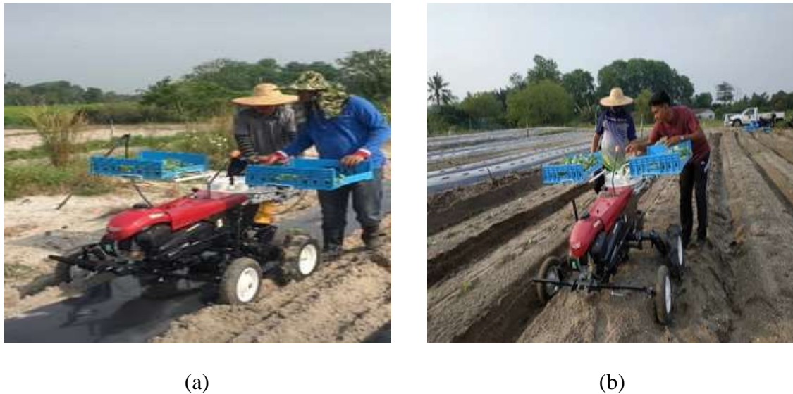
Figure 2. Transplanter operated on planting bed a) with and b) without plastic mulching.
