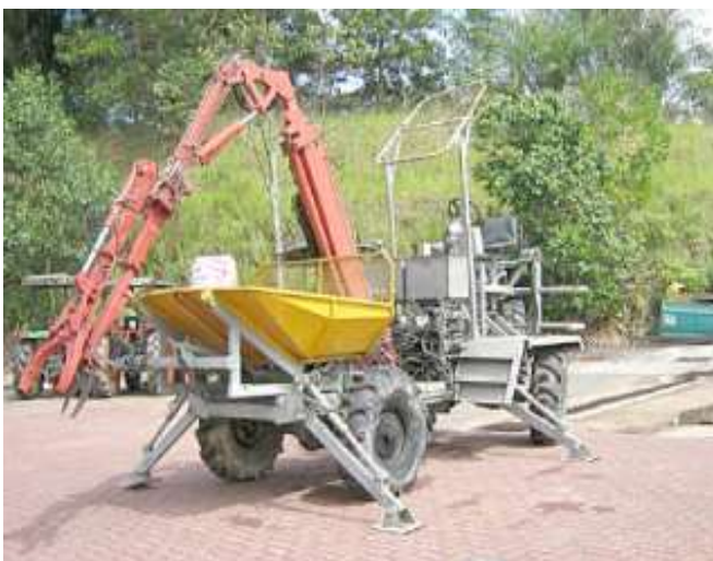
Figure 2. Image and schematic diagram of the harvester manipulator for tall oil palm tress.
