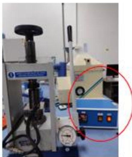
Figure 1. Single Press Hydraulic Machine with temperature controller.
