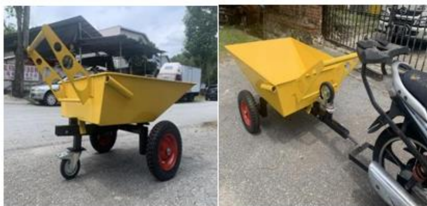
Figure 3. A motorcycle trailer with wheelbarrow functionality.
