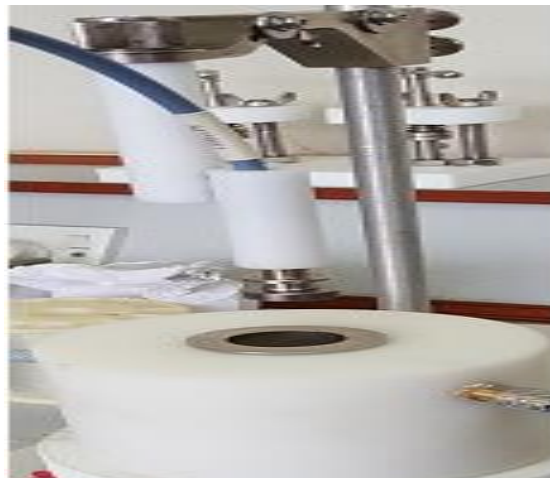
Figure 1. The sample holder and open-ended coaxial-line probe for dielectric properties measurement.
