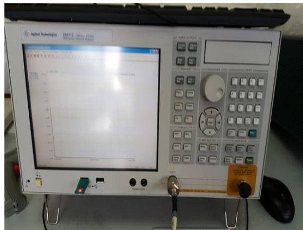
Figure 2. The permittivity of MRQ 76 rice were measured using Agilent E5071C Network Analyser and an open-ended coaxial-line probe
