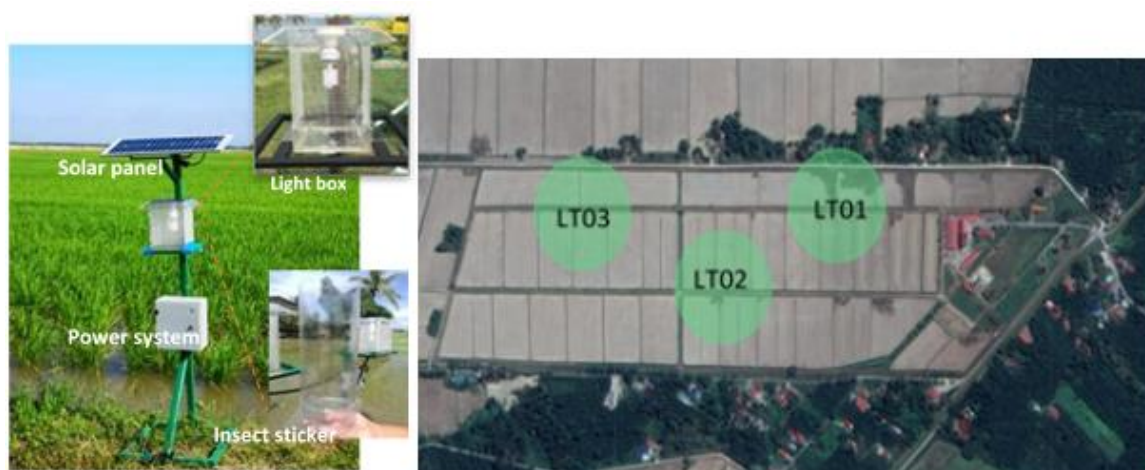
Figure 1. Light trap and location for sampling at MARDI Parit
