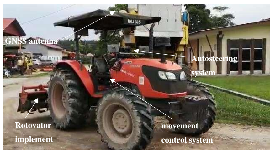
Figure 6. A retrofitted SAPM for land preparation developed by MARDI.
