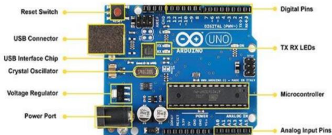
Figure 2. Components of Arduino UNO board
